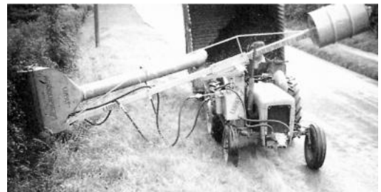
Figure 8: The first flail hedge-cutter, introduced in 1961 greatly reduced hedge-cutting times
